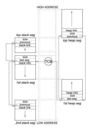
Figure 3: Per thread segment stacks
