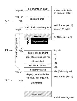
Figure 4: Non-linear stack extension
