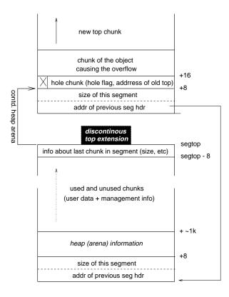
Figure 5: Heap extension
