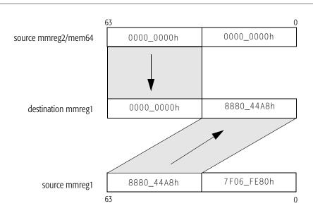
In the functional illustration of the PUNPCKHDQ instruction, the 32-bit value from mmreg1 is stored in the low-order 32 bits of the 64-bit result. The mmreg2/mem64 source operand is set to all zero bits so it can provide zero fill in the high-order 32 bits of the 64-bit result. This is a method that can be used to expand unsigned 32-bit values into unsigned 64-bit operands for subsequent processing that requires higher precision.
