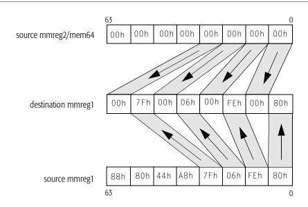
In the functional illustration of the PUNPCKLBW instruction, the 8-bit values from mmreg1 are stored in the low-order 8 bits of the 16-bit result. The mmreg2/mem64 source operand is set to all zero bits so it can provide zero fill in the high-order 8 bits of the 16-bit result. This is a method that can be used to expand unsigned 8-bit values into unsigned 16-bit operands for subsequent processing that requires higher precision.
