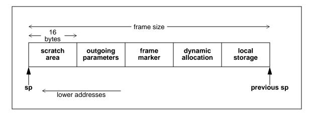
Figure 7-1. Procedure frame
