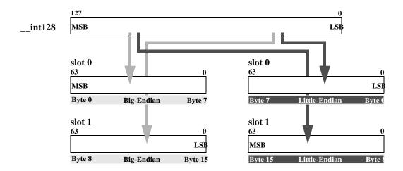
Figure 8-4. Examples of "LSB" Alignment
