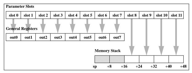
Figure 8-3. Parameter Passing in General Registers and Memory
