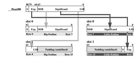
Figure 8-5. Example of "Byte 0" Alignment
