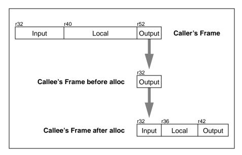
Figure 6-1. Operation of the Register Stack
