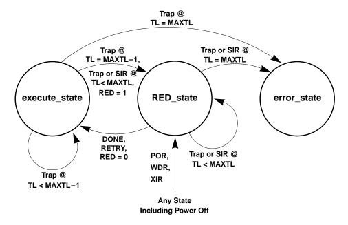
Figure 37—Processor State Diagram
