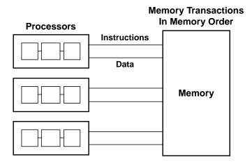
Figure 43—Data Memory Paths: Multiprocessor System
