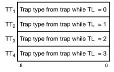
Figure 23—Trap Type Register
