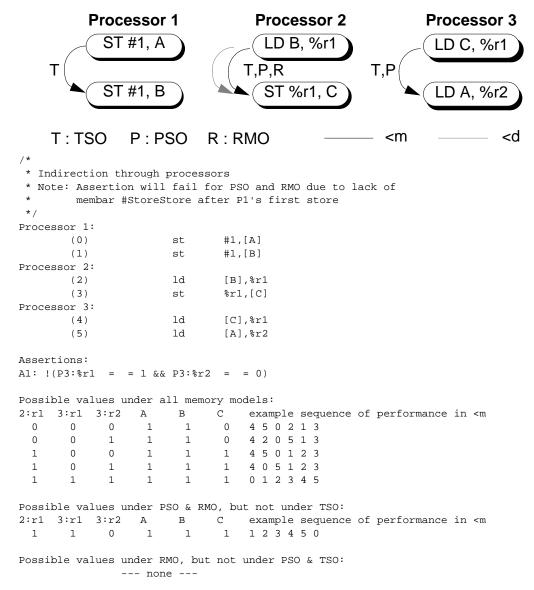
Figure 46—Indirection Through Processors
