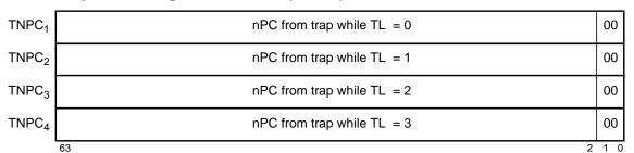
Figure 21—Trap Next Program Counter Register
