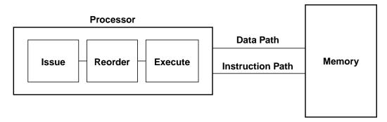
Figure 42—Processor Model: Uniprocessor System
