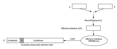
Figure 4-55. Vector Load Element Indexed Operation
